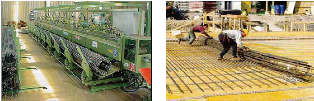
Figure 18: (Left) 3D CAD systems can provide input for reinforcement prefabrication. (Right) Prefabricated reinforcement mats rolled out, decreasing activities on site compared to traditional reinforcement.
